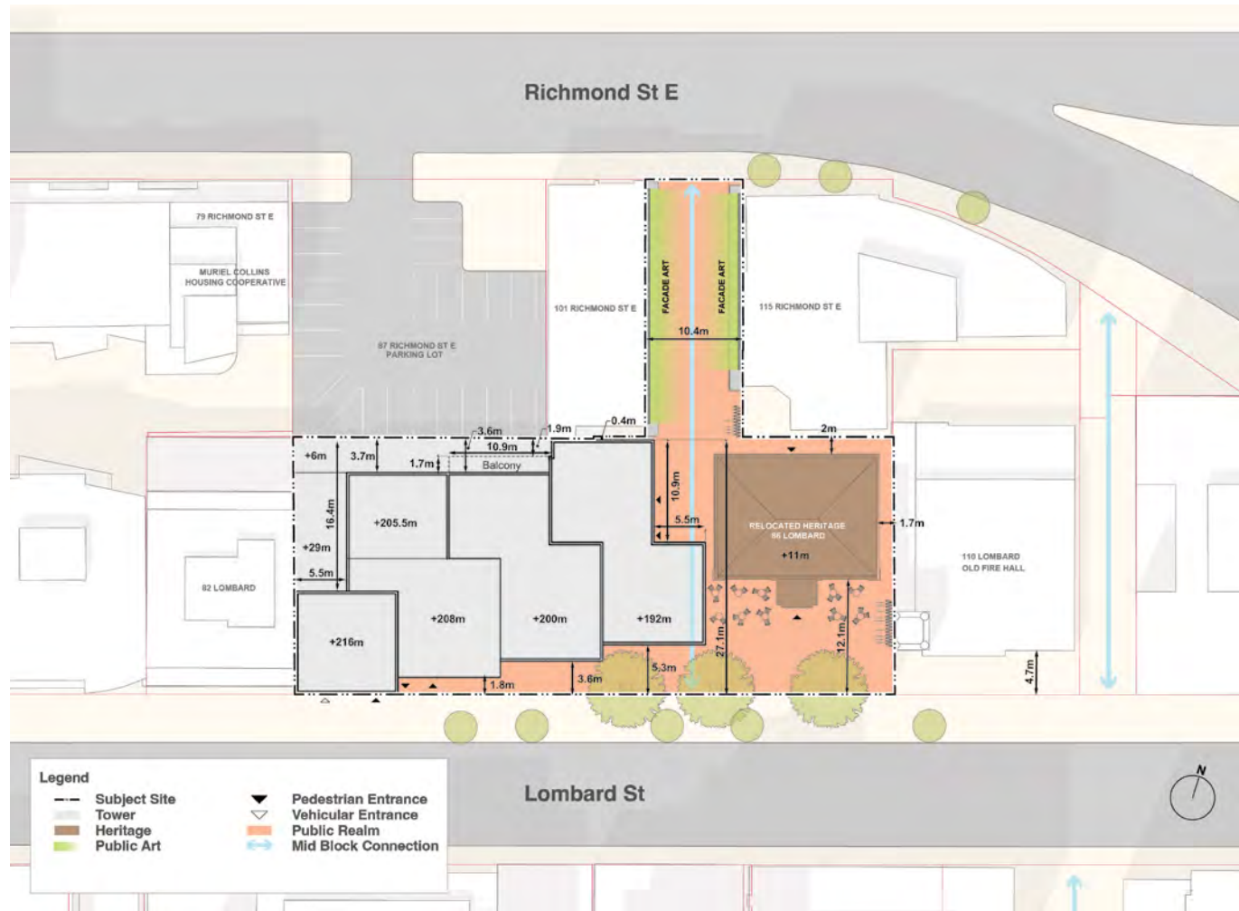
Figure 66. Site Plan with podium setbacks
